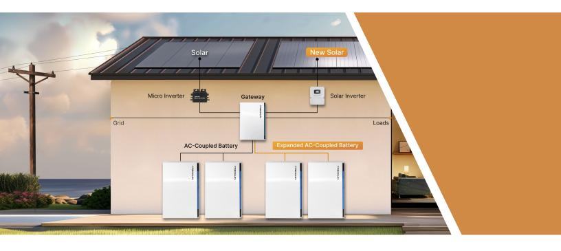
Time-of-use capabilities are a great example of how the FranklinWH system works with the grid. TOU functionality allows homeowners to save on electricity costs by balancing power from the grid, PV system and battery during off-peak hours, and using solar and battery during peak times. By preventing the home from drawing grid power during peak utility rate periods, the battery can pay for itself several times over.
