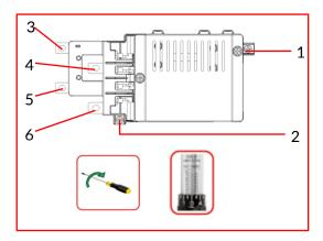
c) Install the metal base of the Smart Circuits Module at the indicated location in the diagram. Use a Phillips screwdriver to tighten the two M4x10 screws at positions 1 and 2 to the recommended torque.
