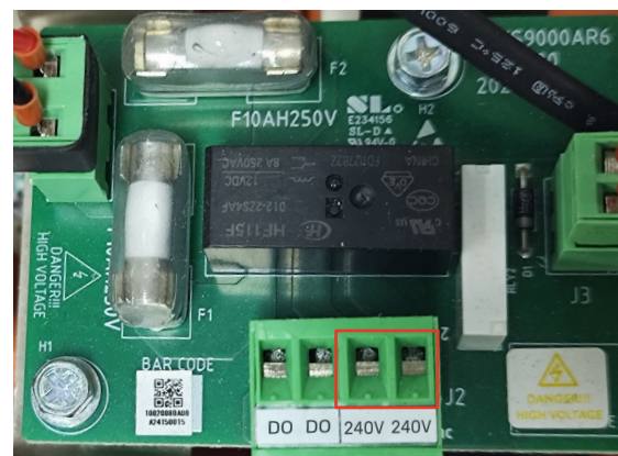
Utility voltage port on the Generator Module
