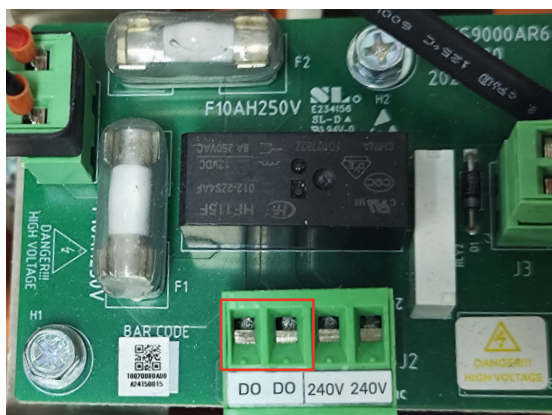
DO/DO port on the Generator Module
