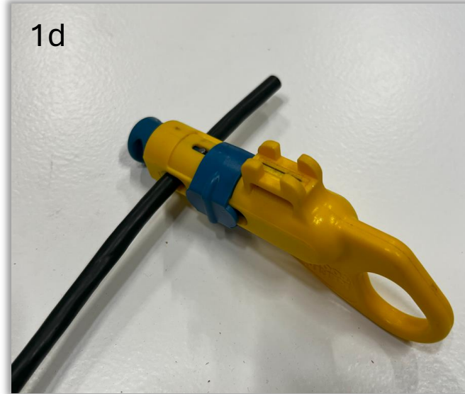
Score the cable jacket at the mark. In this example photo, a Klein VDV110-295 radial stripper is being used.
