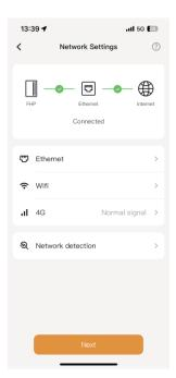
**NOTE:** A Wifi or Ethernet connection is preferred to the 4G cellular network, as 4G is easily affected by the carrier services and weather conditions.
