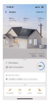
When the system is working normally in on-grid mode and the solar relay has been turned on, if there is still sunshine the solar system will start in 5 minutes.
