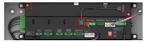
Step 2 Use a Phillips screwdriver to remove two M4 captive screws. Remove the original antenna.
